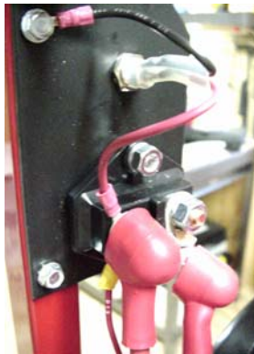
Example of the back side of a push button start switch. Be sure to mark all wires for proper location.
