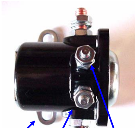
Example of the back side of a push button start switch. Be sure to mark all wires for proper location.
